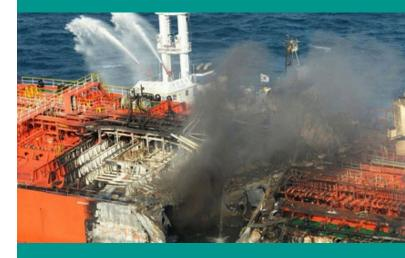
damage, for example, distortion to the ship's steelwork, displacement of items, heat and smoke patterns. Gaining this understanding is critical to interpreting the indicators and thereafter, forensically reconstructing the dynamics of the events.
